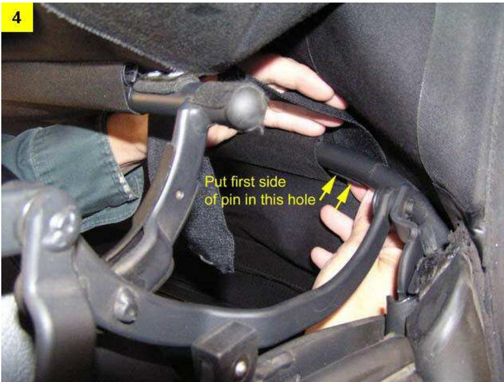
Feed the strap behind the rear support bar from the top, and insert one pin at a time into the rivet holes, starting with the inboard pin. Once the first pin is in, you can swing the U-pin in an arc and the other end will be easier to insert into the other rivet hole.
