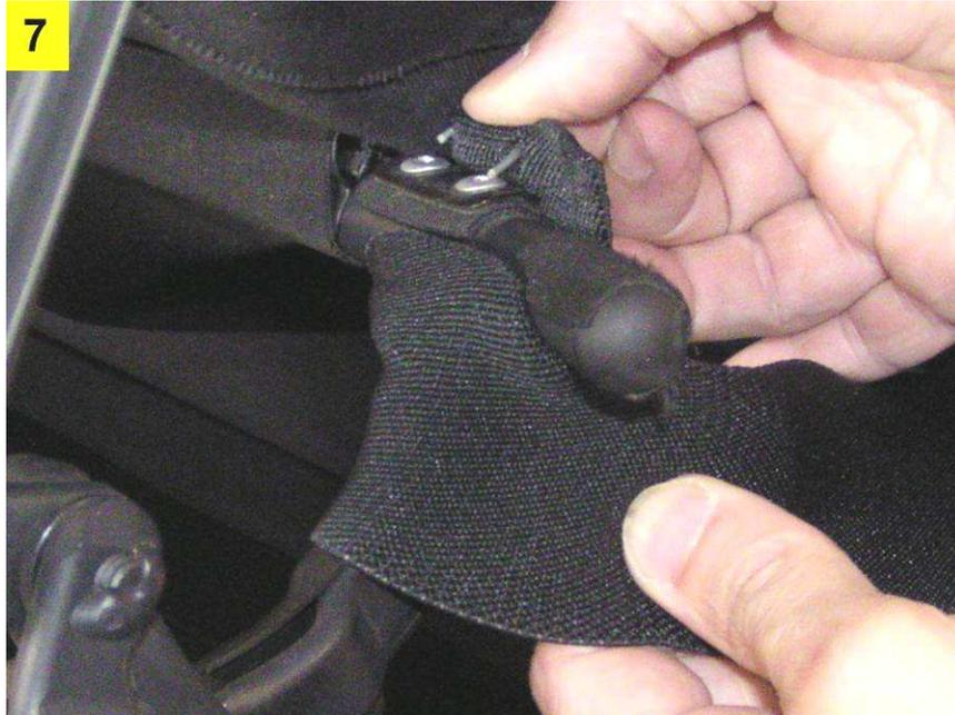
**7. Hook U-pin into front rivet holes.** Stretch the strap with your left hand to give you some slack and insert the U-pin into the rivet holes. While holding the U-pin in place, lift the middle of the strap around and over the end of the bar and position it on top of the rivet plate, so the strap wraps over itself just like the rear did.
