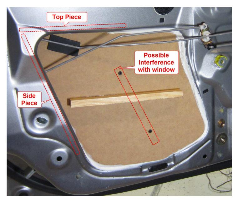
Photo below is a close up of how the Side Piece is mounted and shows the door lock rod going through the slot. I used "Goop" to glue the side and top pieces to the door and clamped them in position until they dried. Goop can be found at Walmart and Home Improvement stores and is marketed under several names, including "Shoe Goop" and "Plumbers Goop", but it's the same stuff.
