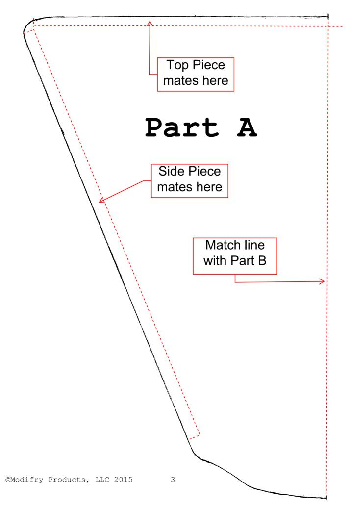
Top Piece mates here This strip tucks behind door opening Part B Bottom edge rests on bottom of door opening
