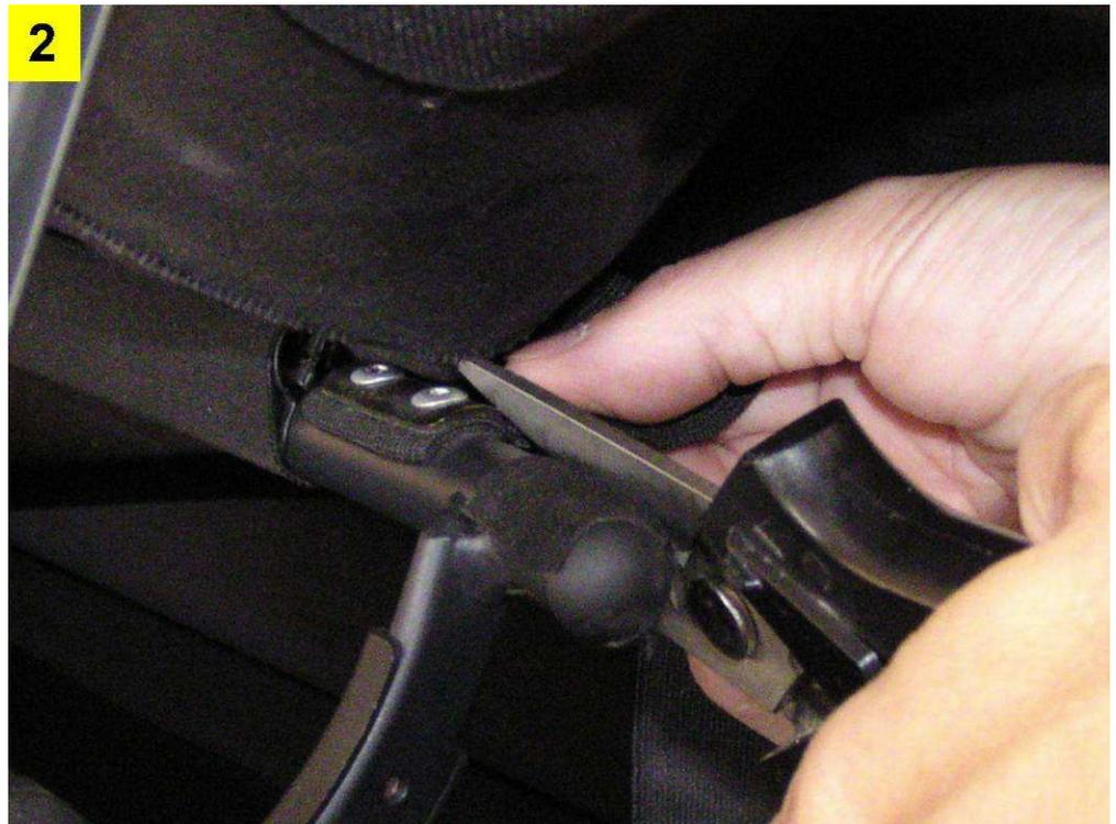
**3. Hold the Modify strap like this.** Make sure the pins are facing you, and the pin closest to the edge of the strap is towards the center of the car. You will insert this pin into the inboard rivet hole. The pins are glued into the strap and should not fall out with normal handling.
