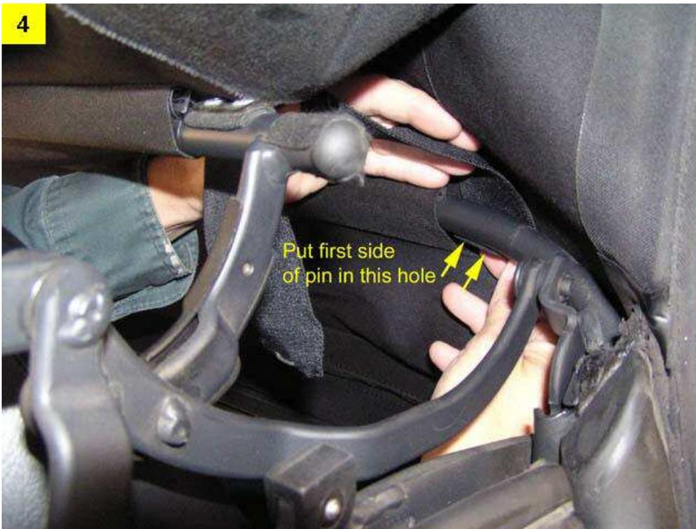
Feed the strap behind the rear support bar from the top, and insert one pin at a time into the rivet holes, starting with the inboard pin. Once the first pin is in, you can swing the U-pin in an arc and the other end will be easier to insert into the other rivet hole.
