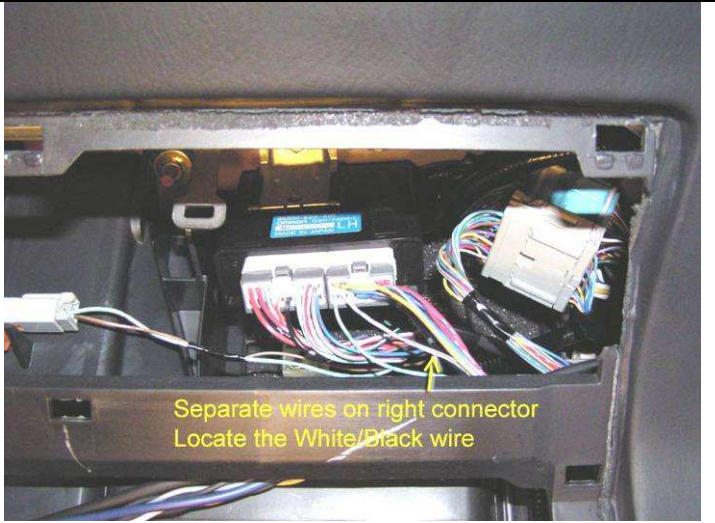
Photo 2 – Convertible Top Module and Speed Signal Wire
