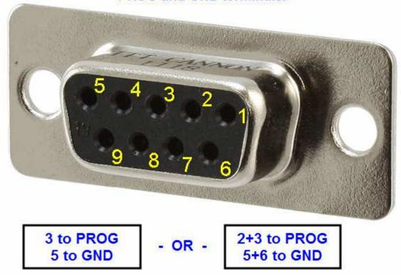
Only 2 wires are needed, but since the wires are very small you may want to double-up as shown to make a sturdier cable.
