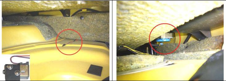
Take a minute to review the next few photos to get a feel for how the SBL mounts to the seat belt assembly. The seat belt assembly has a large square nut on the right side of the bracket and the SBL is designed to fit over the nut. Because you cannot directly see the nut you will have to place the SBL over the nut by feel. Fortunately this not very hard to do and shouldn't take more than a minute or two once you get in position.
