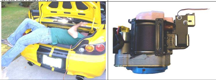
**10. Mount the SBL box and clean up your wiring** – Using the alcohol pad, clean one side of the SBL box and the flat area of the center support. When dry, attach the Velcro strips and position the SBL box so it won't interfere with the access panel when it's installed. Use the provided wire ties to bundle the excess wire and neaten up the installation.
