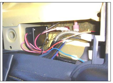
**11. Test the SBL** – Sit in the driver's seat and put on the seat belt. Turn the ignition to the ACC or ON position and press the "A" (Activate) button on the keychain remote. The seat belt should be locked and should not pull out of the reel. Push yourself back into the seat and feed the belt slack into the reel over your left shoulder. The slack should stay there – effectively locking you in the seat.
